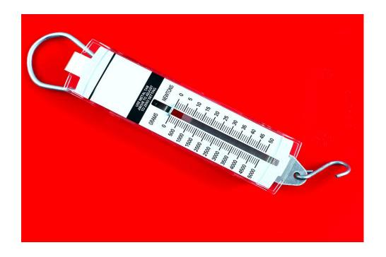
An instrument that measures Earth's gravitational pull on an object
