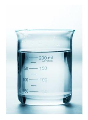
Cylinder shaped glass container used to mix or heat liquids
