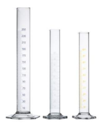
A container used to measure the volume of liquids
