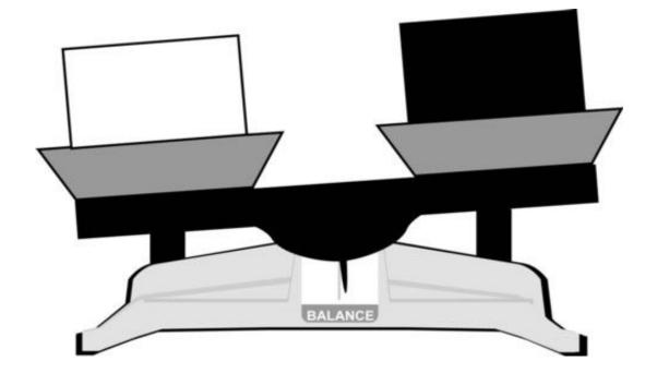
A two-sided instrument that measures the mass of a solid substance
